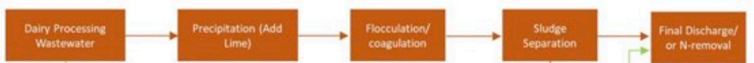
P removal with reduction in lime 40-60%, flocculant (80-85%) and sludge (50%) employing FO-integrated chemical precipitation
