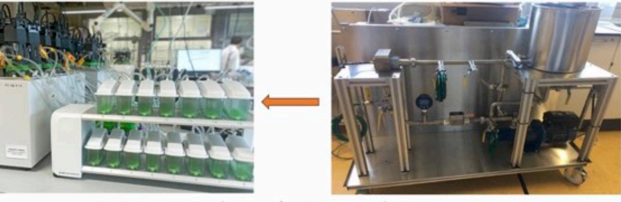
Fig 2: Experimental setup of BMP setup and HC pretreatment
