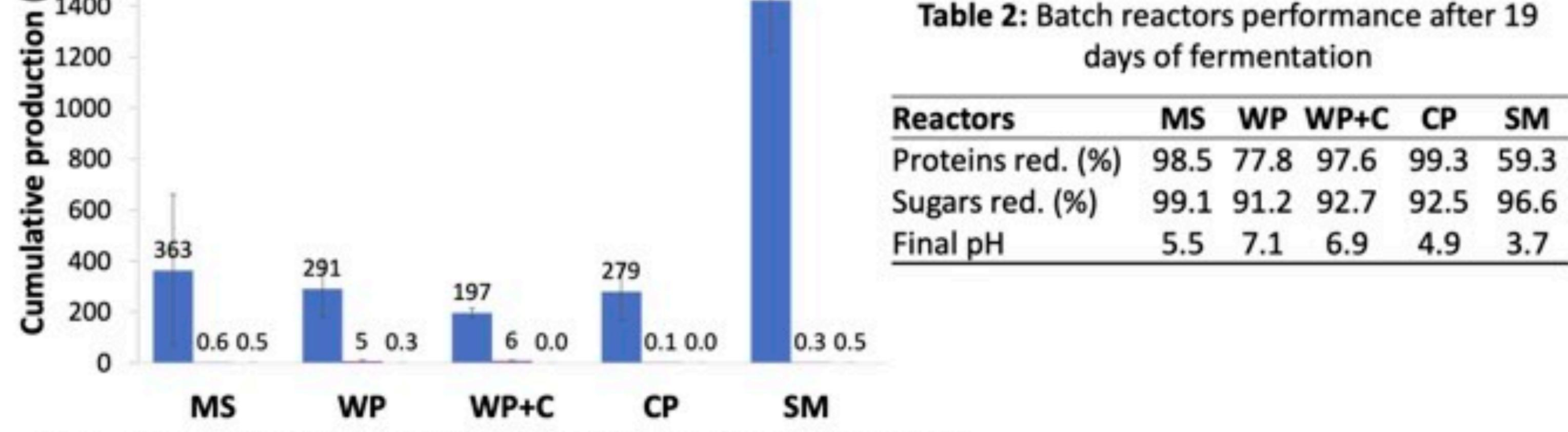
Fig. 2: Biogas, methane and hydrogen production of batch reactors.
